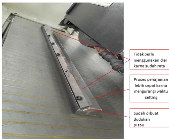
Figure 12. Jig After Modification
