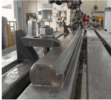
Figure 11. Milling operation using an end mill.
